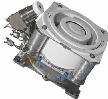
(b) Electric thruster (PPS-1350E)
